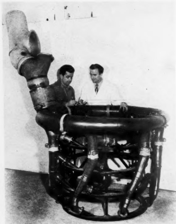
Mr. Hubbell (right) inspects the complete ceramic coated exhaust system that Ryan builds for the engines of the Boeing 377 Stratocruiser.
